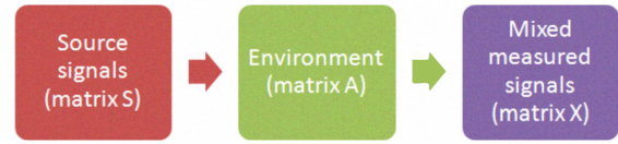
Fig. 1. Schematic representation of the signal mixing process.
