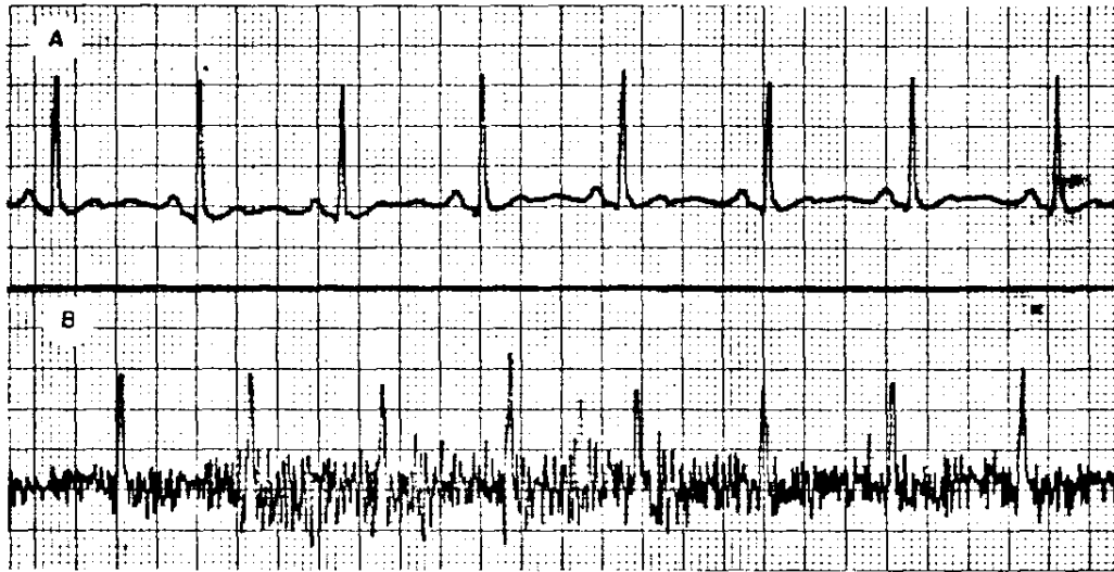
FIG. 2. Comparison of EKG of a subject at rest and performing isometric exercises involving thoracic muscles. Measured with Biocom Model 368 EKG telemetry system. Unfiltered. Electrode location: manubrium to rib in V5 position.
