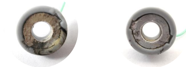
Electrode with layer of oxide;
